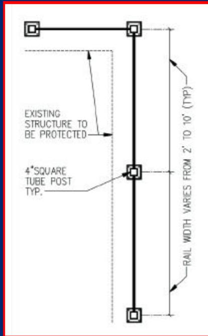
**Rail Sections** - shall be made from 12 gauge steel and shall meet ASTM requirements.
